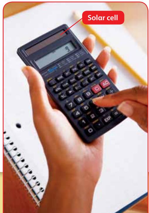
The small, flat solar cell can change solar energy into electricity to run a calculator.
