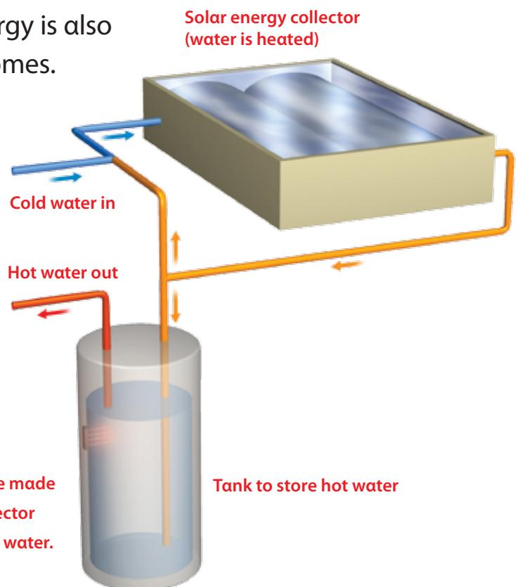
Passive solar water heaters are made of two main parts: a solar collector and a tank to store the heated water.
