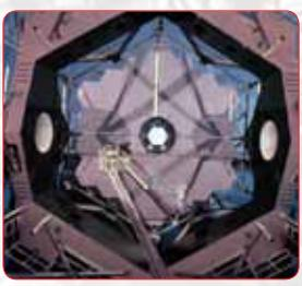
Each of the twin Keck telescopes has a 10-meter system of mirrors. They are the world's largest optical telescopes.
