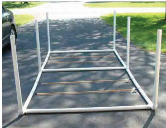
Figure 2: construction of the base.
